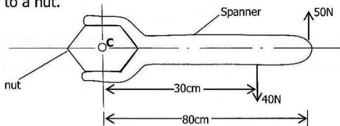
What is the turning effect of the spanner due to the two forces about c, the centre of the nut?
