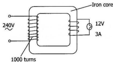
Assuming that the transformer is ideal, what is the number of turns in the output coil and the value of the input current?
